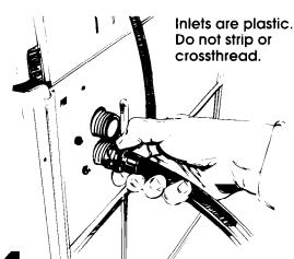
Attach hose to bottom inlet valve opening first; then second hose to top inlet. Tighten couplings by hand. Then use pliers to make an additional two-thirds turn.
